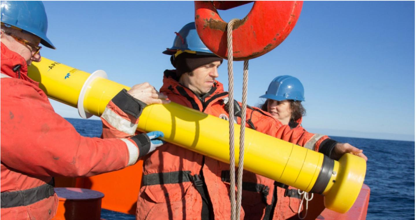
*Aboard the N.B. Palmer research vessel, marine technician MacKenzie Haberman assisted with the launch of a profiling float in the Southern Ocean, which remotely monitors ocean conditions.*
